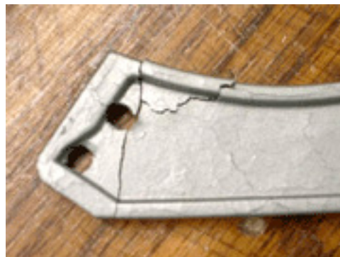
This is the damage as the brackets expand and disintegrate.
