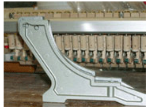
YC Inner Brackets (old behind new) showing the dimensional instability and degree of change.
